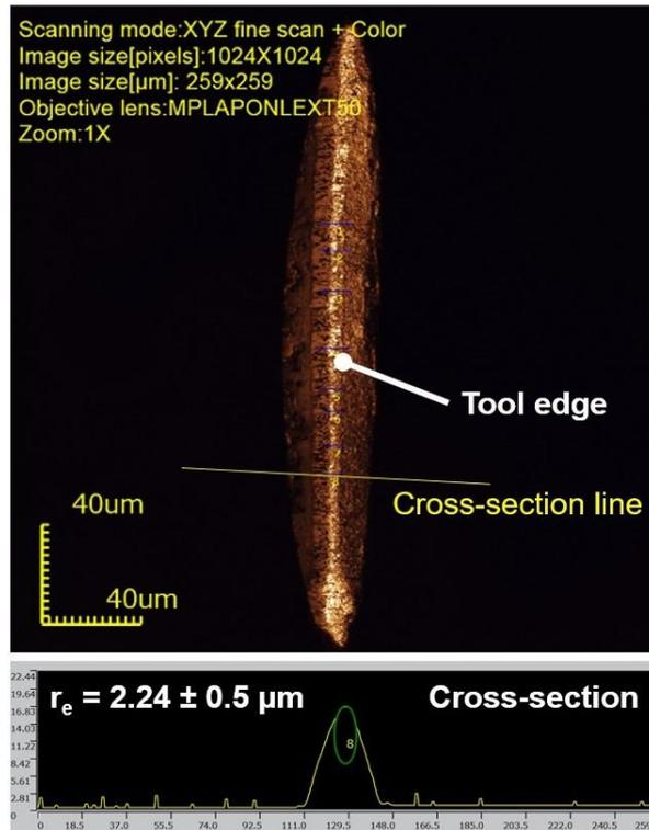
**Figure 2.** Edge radius measurement by 3D laser microscopy.
