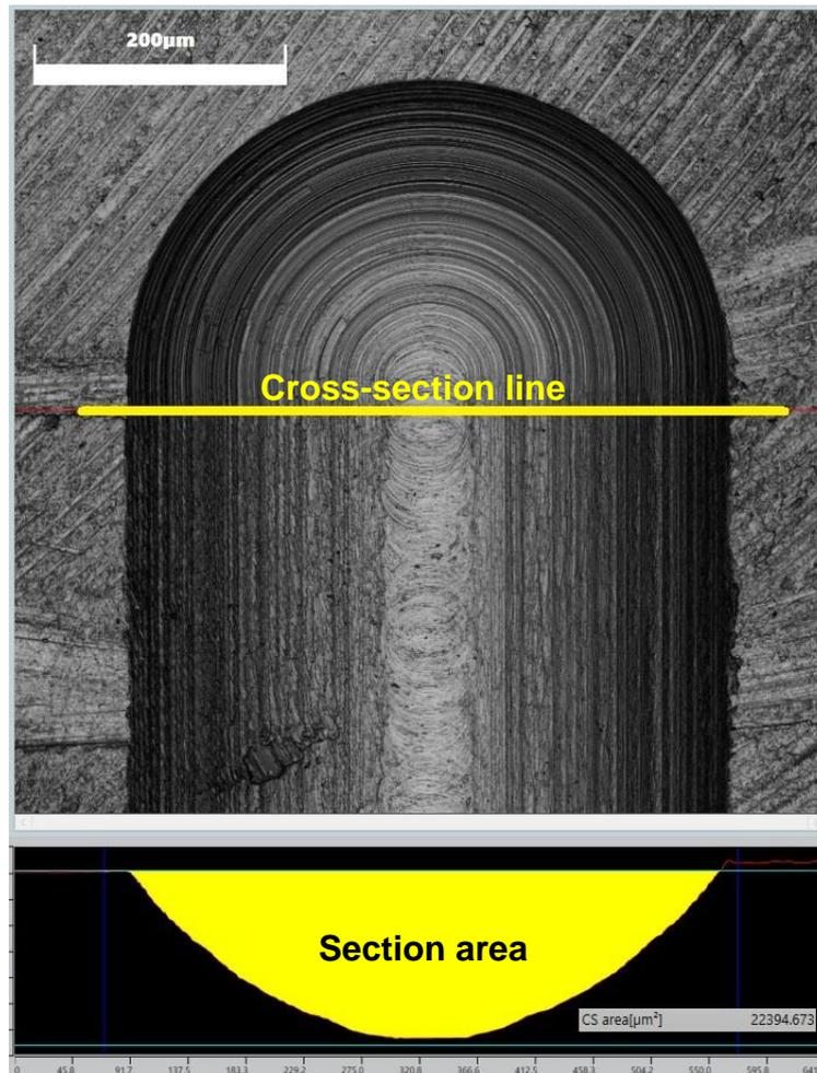
**Figure 3.** Microchannels section area measurement by 3D laser microscopy.
