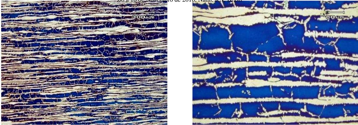
**Figure 9: Microstructure of the UNS 32205 base material. (Modified Behara)**
