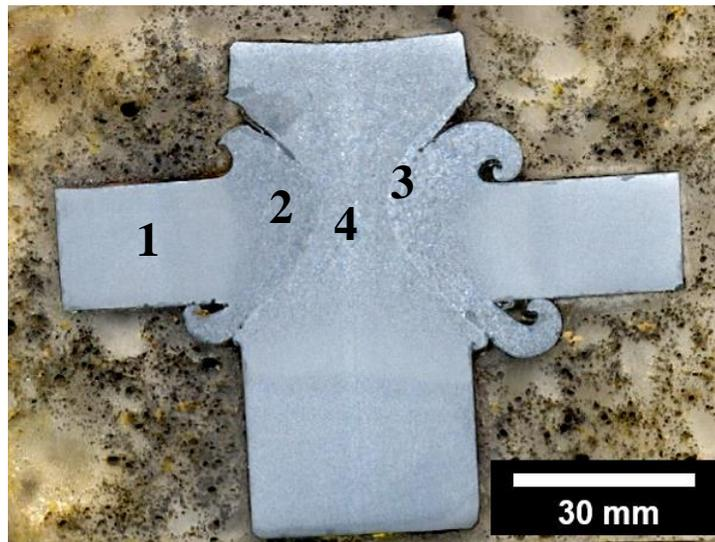
**Figure 5: Macrograph of the weldment performed in ASTM A36 steel and the subsequent analyzed regions.**
