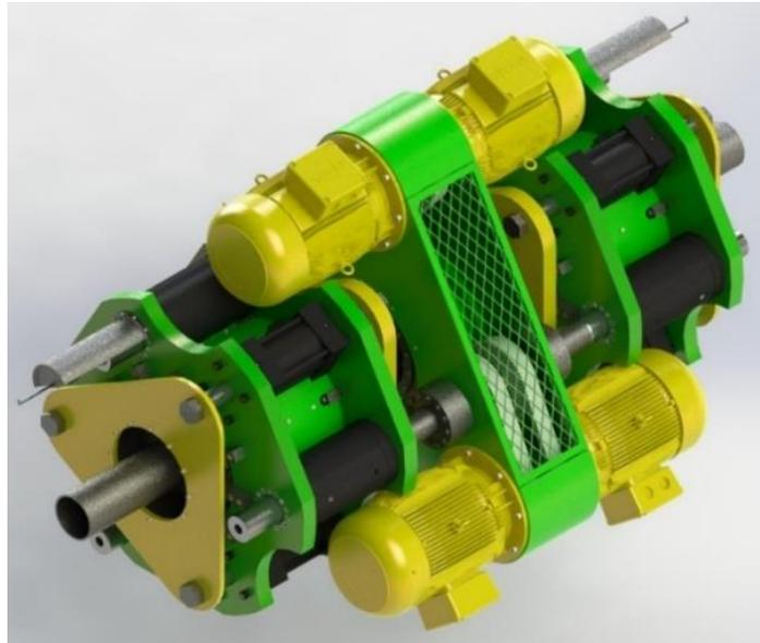
**Figure 2: MASF 1500 equipment for friction welding of pipelines located at LAMEF.**
