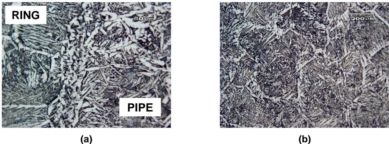
**Figure 7: (a) Microstructure on the interface region between pipe and ring - Region 3. (b) Microstructure of the TMAZ of the ring – Region 4. (Nital 2%)**
