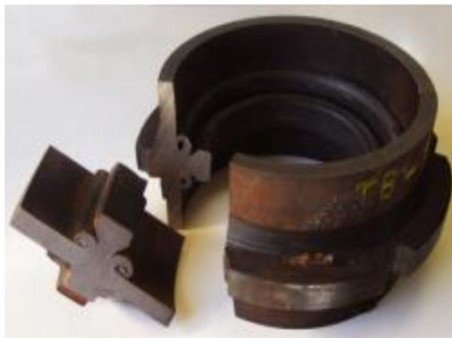
**Figure 4: Weldment with consumable rotatory ring performed in MASF 1500.**
