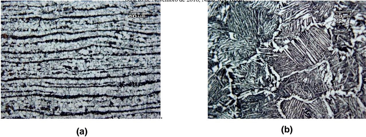
**Figure 6: (a) Microstructure of the ASTM A36 base material – Region 1. (b) Microstructure of the TMAZ of the pipe – Region 2. (Nital 2%)**
