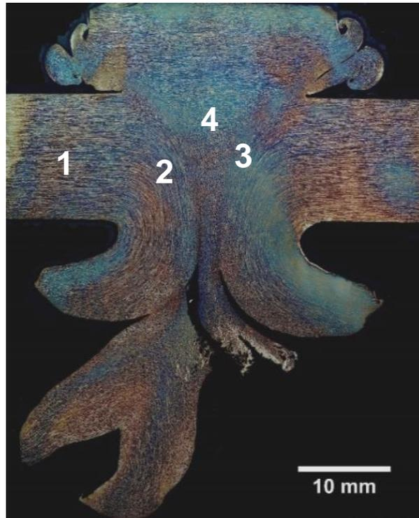
**Figure 8: Macrograph of the weldment performed in UNS 32205 steel and the subsequent analyzed regions.
