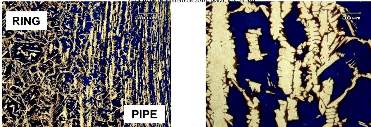
Figure 11: Microstructure on the interface region between pipe and ring. (Modified Behara)
