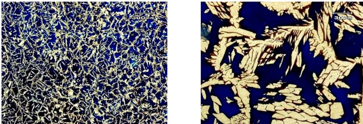
Figure 12: Microstructure of the TMAZ of the ring (Modified Behara)
