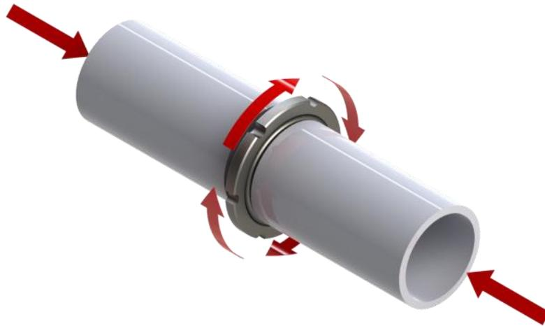
**Figure 1: Schematic illustration of the friction welding process with rotatory ring for pipelines [12].**
