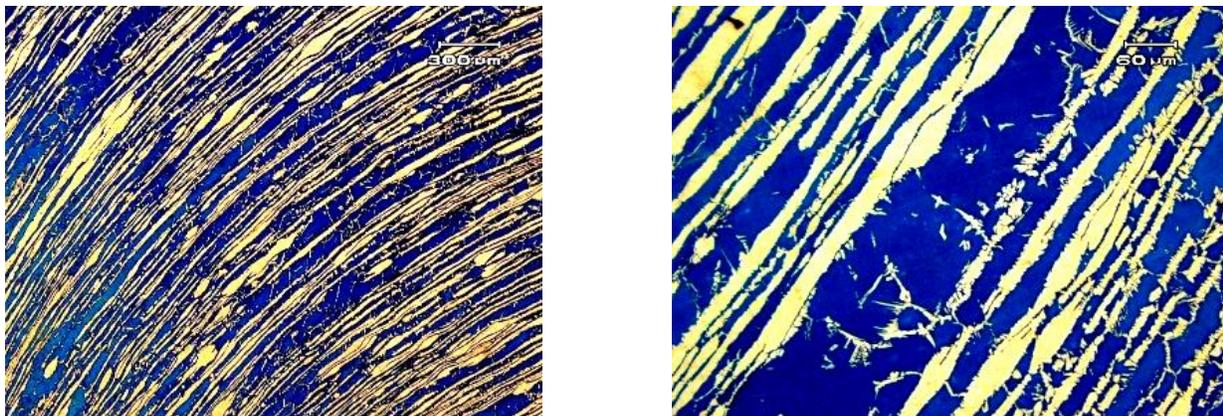
**Figure 10: Microstructure of the TMAZ of the pipe. (Modified Behara)**
