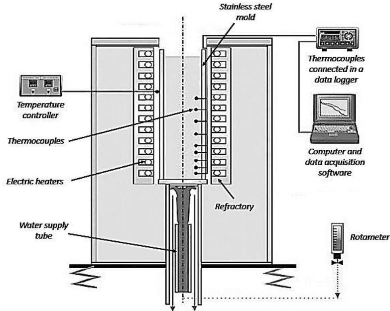
**Fig. 1.** Directional solidification system for transient heat flow conditions and the devices used to monitor solidification.
