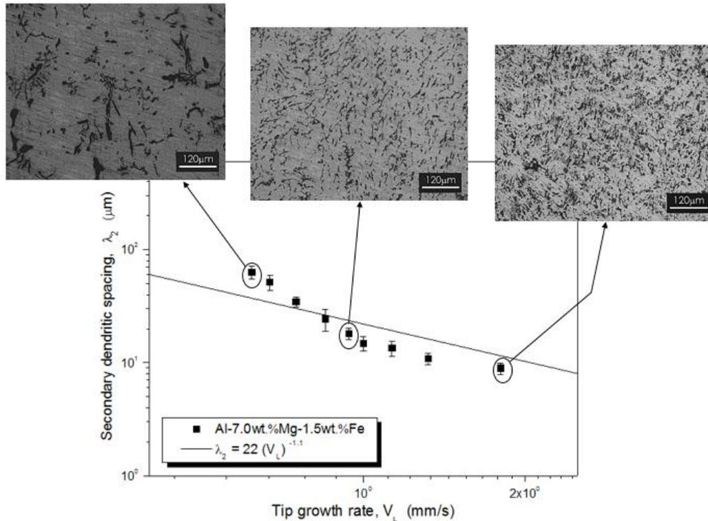
**Fig. 4.** Secondary dendritic spacing ( $\lambda_2$ ) as a function of tip growth rate ( $V_L$ ) for a Al-7.0wt.%Mg-1.5wt.%Fe alloy. Details of microstructure evolution are given by longitudinal optical images in different positions of ingot.
