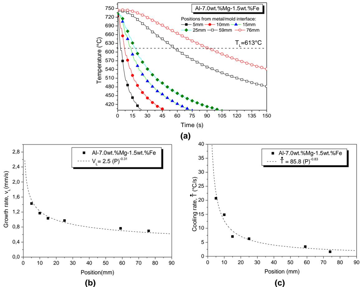
**Fig. 3.** (a) Typical experimental thermal responses of thermocouples at six locations in casting from the cooled surface for the Al-Mg-Fe alloy sample; (b) growth rate and (c) cooling rate against position.  $T_L$  is the *liquidus* temperature.
