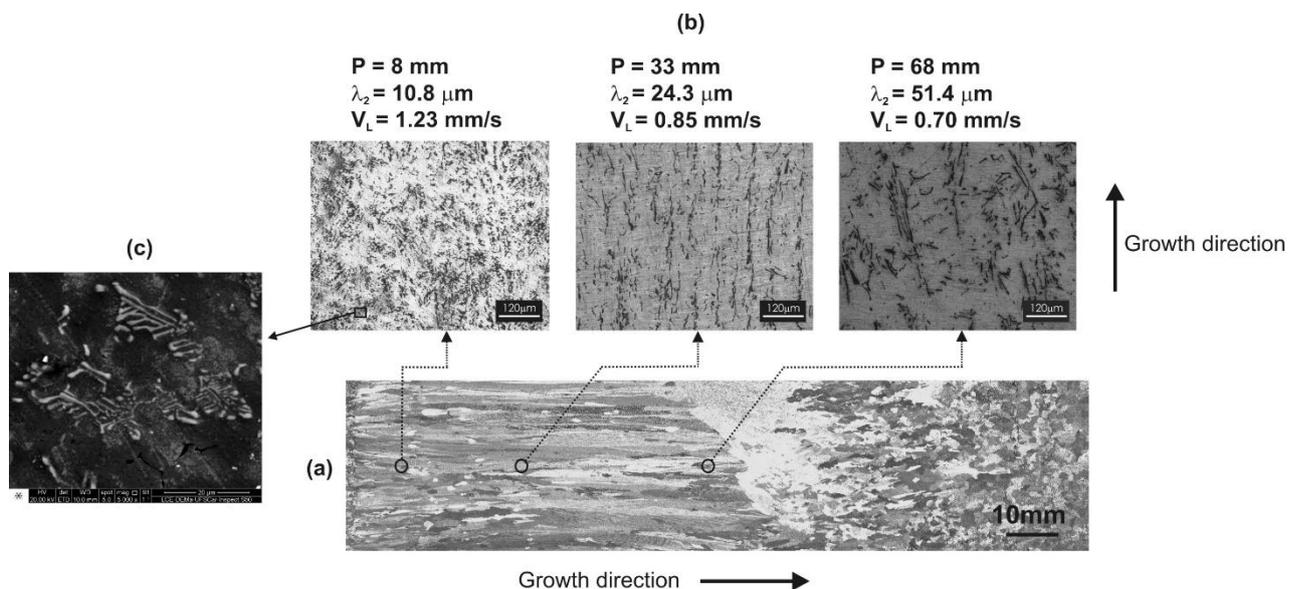
**Fig. 2.** (a) Directionally solidified macrostructure of the Al-7.0wt.-%Mg-1.5wt.-%Fe alloy casting and (b) longitudinal as-cast microstructures for different positions with
