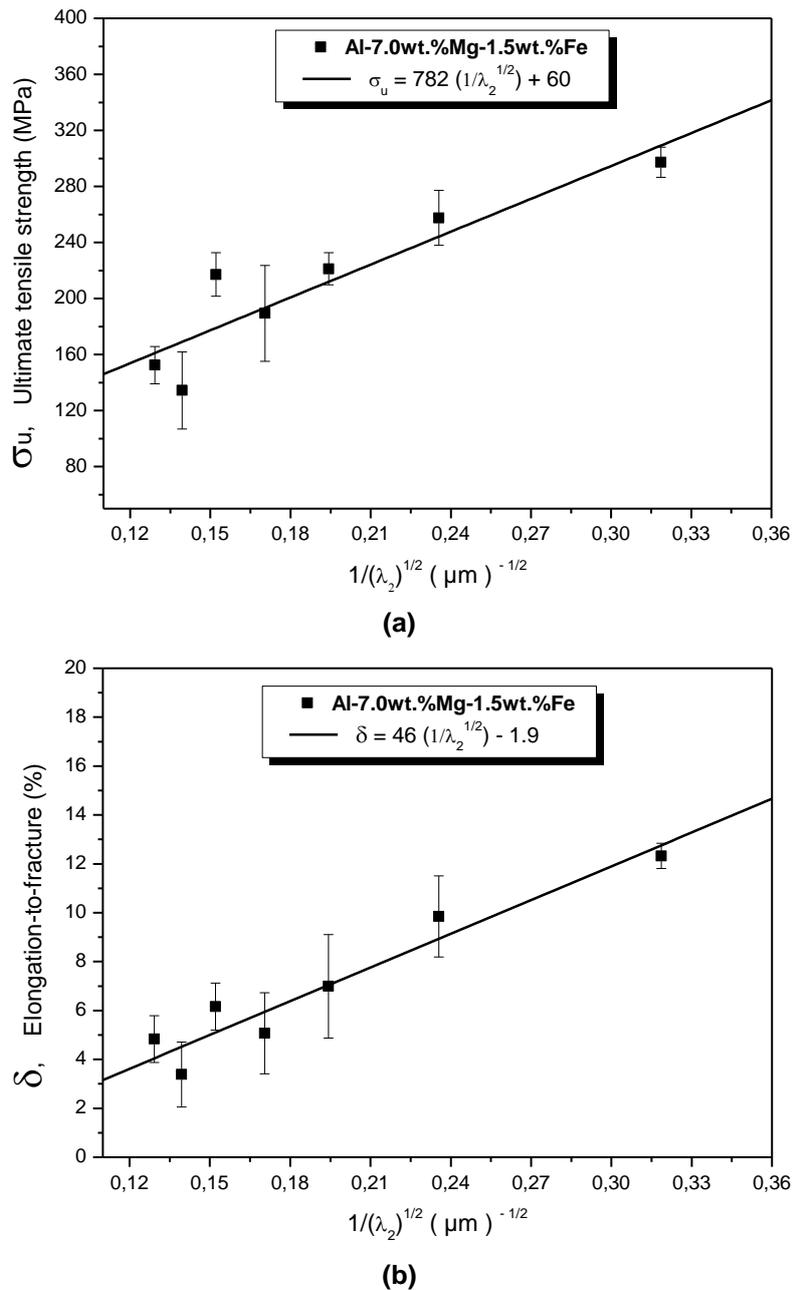
**Fig. 5.** Ultimate tensile strength ( $\sigma_u$ ) and Elongation ( $\delta$ ) as a function of secondary dendritic spacing ( $\lambda_2$ ) for a Al-7.0wt.%Mg-1.5wt.%Fe alloy.
