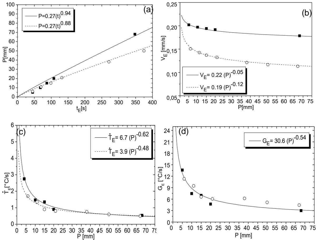
Figure 2. Graphs showing (a) Displacement of eutectic front; (b) eutectic growth rate; (c) eutectic cooling rate; and (d) thermal gradient along the Al-15wt.%Si and Al-18wt.%Si alloys. ■ Al-15wt.%Si; ○ Al-18wt.%Si.
