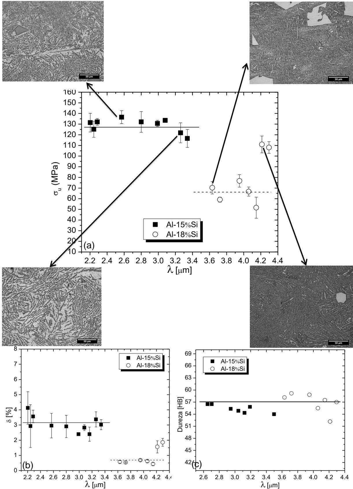
Figure 4. Tensile mechanical properties of the Al-15wt%Si and Al-18wt%Si alloys: (a) tensile strength; (b) elongation-to-fracture; and (c) Brinell Hardness as a function of the eutectic spacing ( $\lambda$ ) ■ Al-15%Si; ○ Al-18%Si.
