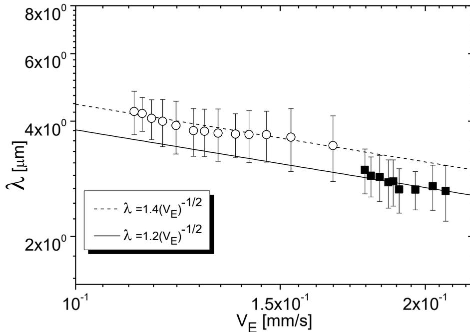
Figure 3. Eutectic spacing along the directionally solidified Al-15wt%Si and Al-18wt%Si alloys as a function of the eutectic growth rate. ■ Al-15%Si; ○ Al-18%Si.
