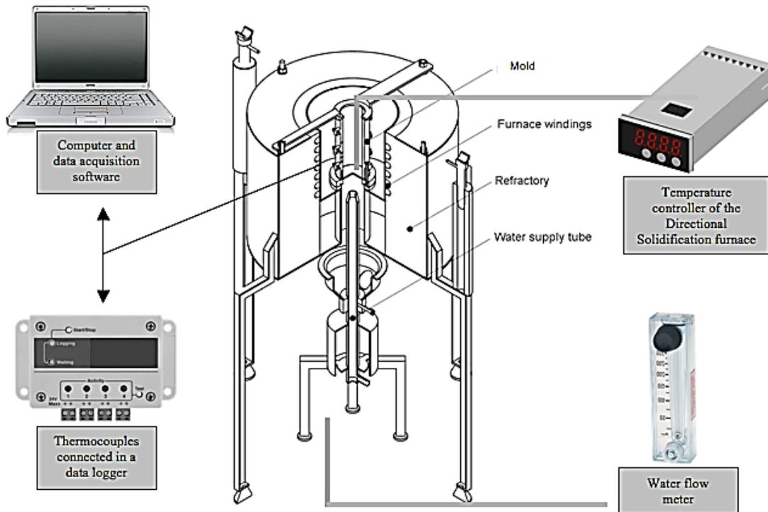
Figure 1. Unidirectional solidification system for transient heat flow extraction coupled with the necessary devices.
