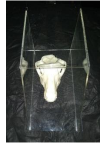
Figure 14 – Canine skull simulator made in a 3D printer, placed inside the positioner. Source: author.
