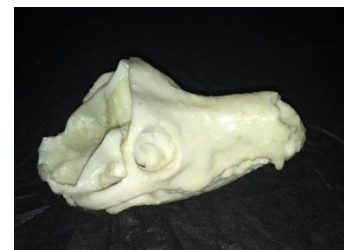
Figure 12 – Canine skull simulator made in a 3D printer (side view). Source: author.
