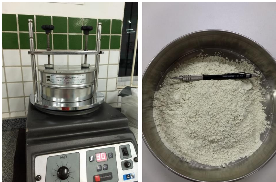
Figure 3. ABNT mesh sieve No. 200 (left), and final visual appearance of the residue (right).
