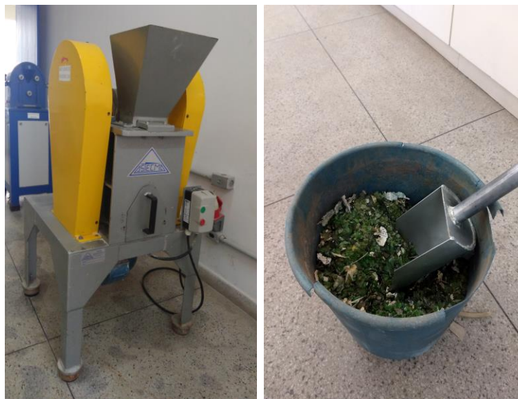
Figure 1. Jaw crusher used (left), and crushed residue (right).
