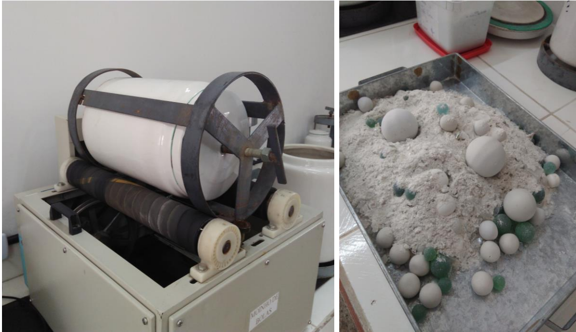
Figure 2. Ball mill used (left), and ground residue (right).
